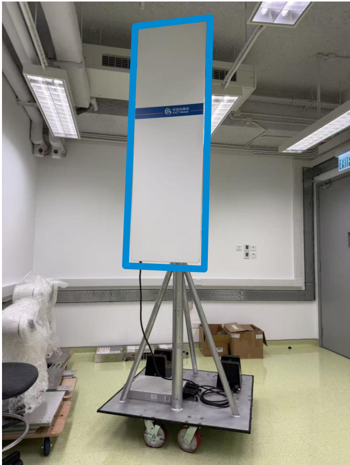
6G Massive MIMO BS 1024 antennas, 128 ports
